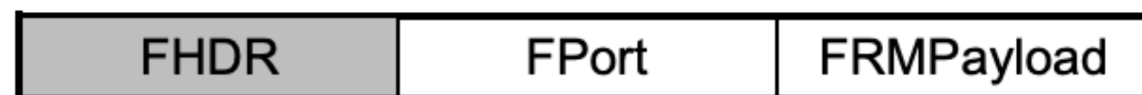
Figure 7: MAC payload structure
